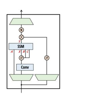
The full model consists of 64 Mamba 2 SSM blocks, each of the which consist of the following layers:
